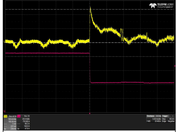
Figure 8: LCM1000L-T Transient Response - Vo Deviation 100% to 50% load change 1A/uS slew rate Vin = 90Vac Ch 1: Vo Ch 2: Io
