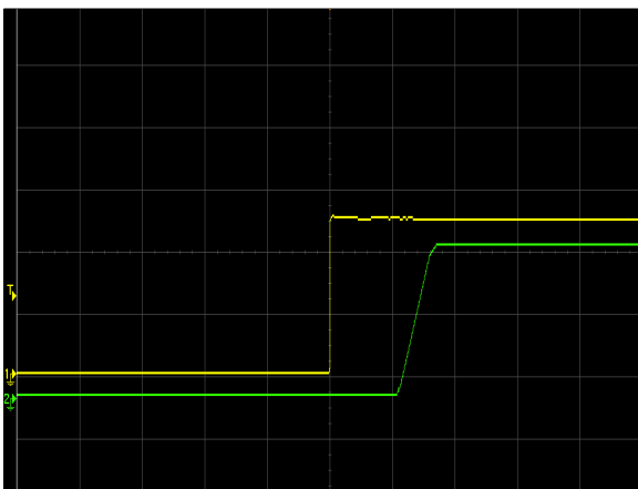
Figure 3: NDQ900-48S12B-6LI Output Voltage Startup by Power On Vin = 50 Vdc Load: I o = 73.7 A Ch 1: V in (20V/div) Ch 2: V out (5V/div) (50mS/div)
