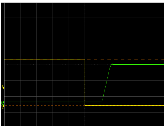
Figure 5: NDQ900-48S12B-6LI Output Voltage Startup by Remote On Vin = 50 Vdc Load: I o = 73.7 A Ch 1: Remote on (1V/div) Ch 2: V out (5V/div) (50mS/div)
