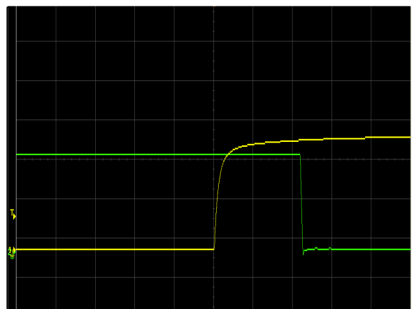
Figure 6: NDQ900-48S12B-6LI Output Voltage Startup by Remote Off Vin = 50 Vdc Load: I o = 73.7 A Ch 1: Remote off (1V/div) Ch 2: V out (5V/div) (10mS/div)
