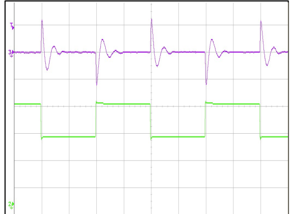
Figure 8: ADQ600B-48S12B-6LK Transient Response (2mS/div) 50%~75%~50% load change, 1A/uS slew rate, Vin = 48Vdc Ch 2: Io (10A/div) Ch 3: Vo (200mV/div)
