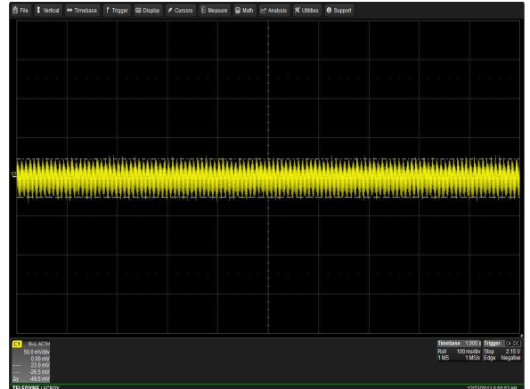
Figure 10: LCM1500L-T-4 Ripple and Noise Measurement Vin = 115Vac Load: I_o = 125A (12V), I_{sb} = 2A (5V) Ch 1: Vo
