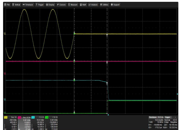
Figure 15: LCM1500N-T-4 Hold-up Time Vin = 264Vac / 60Hz / 0° Load: lo = 100A (15V), Isb = 2A (5V) Ch 1: Vin Ch 2: Vsb Ch 3: Vo Ch 4: G_DCOK_C
