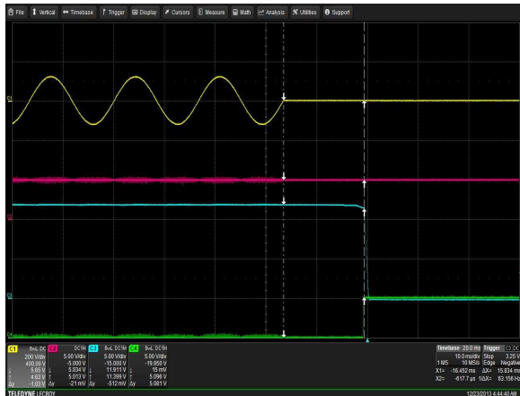
Figure 3: LCM1500L-T-4 Hold-up Time Vin = 90Vac / 47Hz / 0° Load: lo = 125A (12V), Isb = 2A (5V) Ch 1: Vin Ch 2: Vsb Ch 3: Vo Ch 4: G_DCOK_C
